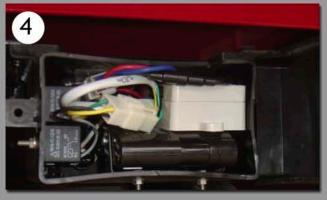
4. Carefully place the new Wireless Receiver on top of the brake controller in the Black Box.
