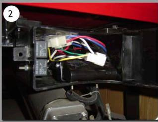
Locate the preinstalled 4 pole connector inside the Black Box, which has yellow, green, black, and white wires connected to it.
