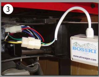
3. Connect the Wireless Receiver plug to the 4 pole connector in the Black Box. Be sure to align and match the colored wires correctly. Push the connectors together until it clicks.
