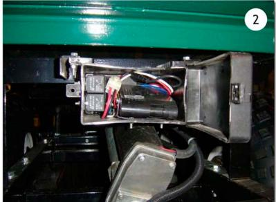
3. Gently remove the relay section, carefully feeding additional wire from the back of the Black Box so you have more area to work.
