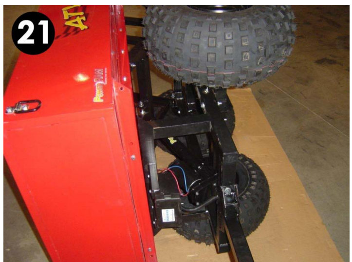
21. With the help of 2 people, carefully turn trailer over onto tires. Be careful not to damage tailgate pins or D-rings.
