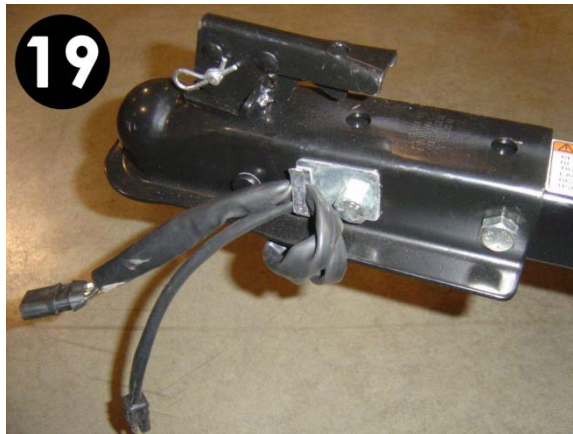
19. Place tongue wires in hook on coupler.
