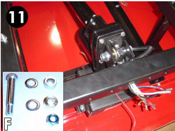
11. Install lift, with motor closest to frame. Be sure to use the shorter spacers from package labeled F.
