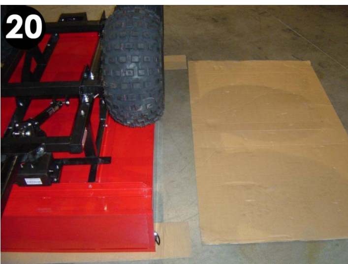
20. Use cardboard and position as shown above to protect sides and wheels.
