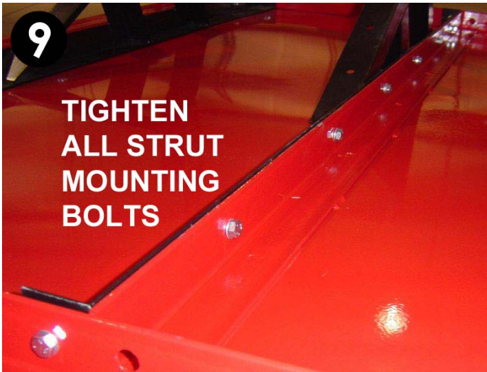
9. Tighten bolts that join bed and sub frame struts from Step 4.
